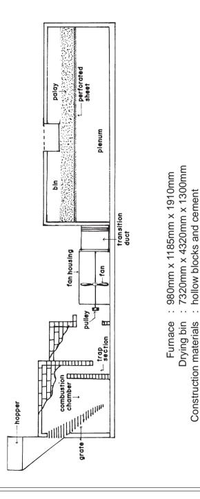
Equipped with several windows for grain unloading. False floor is made of gauge #22 perforated sheets with 2.44 mm diameter holes and supported by 4cm x 8 cm wooden frame.
