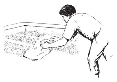
3. After loading, level the palay to have uniform air distribution.
