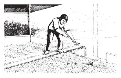
4. Load rice hull at the hopper of the furnace.
