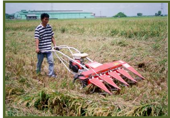
Reciprocating cutter-bar reaper
