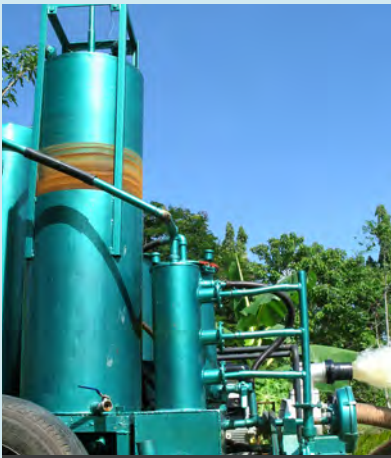
Rice hull Gasifier
