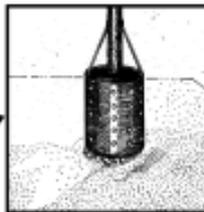
3. Place 12-14 sacks of rice hull around the carbonizer or until it reaches the chimney at 1 meter high. This is to maximize burning time and effort to make more CRH during carbonization than putting a minimum of 3 sacks rice hull around the carbonizer per batch.
