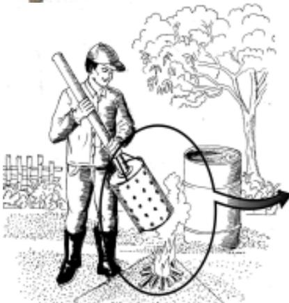
2. Cover the fire with an open-type carbonizer. *(see p 10)*
